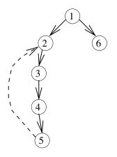
Figure 5.12: DFS tree of a graph containing two articulation vertices (namely 1 and 2). Back edge (5, 2) keeps vertices 3 and 4 from being cut-nodes. Vertices 5 and 6 escape as leaves of the DFS tree
