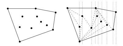
Figure 4.1: The convex hull of a set of points (1), constructed by left-to-right insertion.
