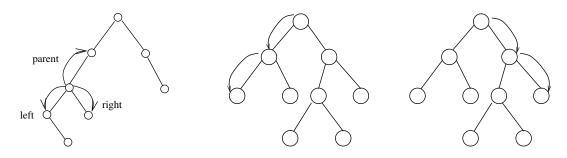
Figure 3.3: Relationships in a binary search tree (left). Finding the minimum (center) and maximum (right) elements in a binary search tree
