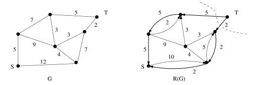
Figure 6.13: Maximum s - t flow in a graph G (on left) showing the associated residual graph R(G) and minimum s - t cut (dotted line near t)
