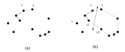
Figure 6.4: Where Kruskal's algorithm goes bad? No, because  $d(v_1, v_2) \ge d(x, y)$
