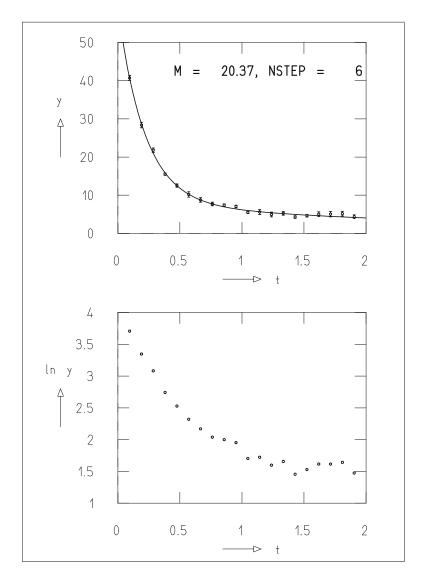
**Fig. 9.7:** Measured values with the fitted sum of two exponential functions (*above*); logarithm of the measured values (*below*).
