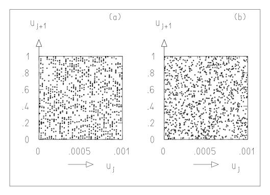
**Fig. 4.3:** Scatter plots of number pairs (4.5.4) from (**a**) a MLC generator and (**b**) a combined generator. The methods DatanRandom.mclg and DatanRandom.ecuy, respectively, were used in the generation.
