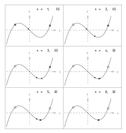
**Fig. 10.7:** Stepwise bracketing of a minimum with the combined method of Brent. The initial interval (*large circles*) is reduced with each step (*small circles*). Steps are carried out according to the golden section (GS) or by quadratic interpolation (QI).
