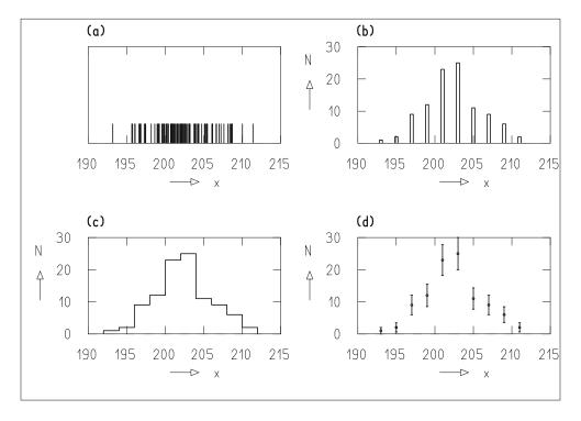
**Fig. 6.1:** Representation of the data from Table 6.1 as (**a**) a one-dimensional scatter plot, (**b**) a bar diagram, (**c**) a step diagram, and (**d**) a diagram of measured points with error bars.
