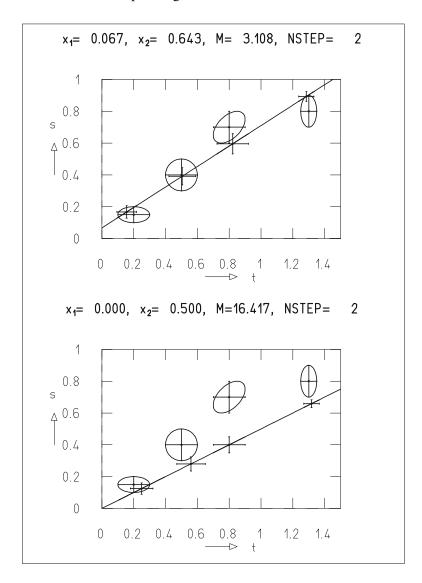
**Fig. 9.14:** Constrained measurements. The hypothesis was tested whether the true values of the measured points, indicated by their covariance ellipses, lie on the line  $s = x_1 + x_2t$ . With the numerical values of M, a  $\chi^2$ -test with four degrees of freedom can be carried out. Shown as well are the improved measurements, which lie on the line, and their errors.
