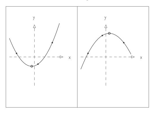
**Fig. 10.2:** Parabola through three points (*small circles*) and its extremum (*large circle*). In the *left figure* there is a minimum, and on the *right* a maximum.
