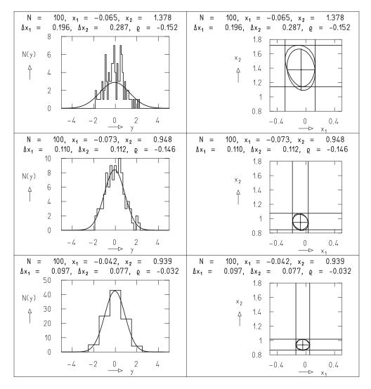
**Fig. 10.19:** Determination of the parameters  $x_1$  (mean) and  $x_2$  (width) of a Gaussian distribution by minimization of a weighted sum of squares. The histograms on the *left* are the same as in Fig. 10.18. The fit results and errors, covariance ellipses, and confidence regions are represented as in Figs. 10.17 and 10.18.
