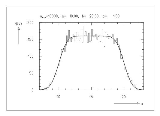
**Fig. G.7:** A histogram of 10 000 random numbers, each of which is the sum of a uniformly distributed random number and a normally distributed random number. The curve corresponds to the convolution of a uniform and a normal distribution.
