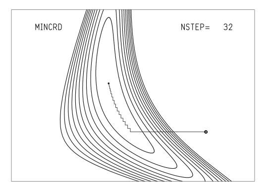
**Fig. 10.10:** Minimization along the coordinate directions. The starting point is shown by the *larger circle*, and the end by the *smaller circle*. The *line* shows the results of the individual steps.
