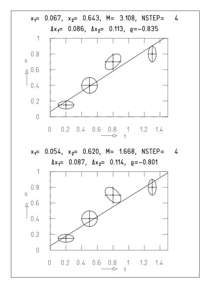
**Fig. 9.12:** Fitting a line to four measured points in the (t, s) plane. The points are shown with measurement errors (in t and s) and covariance ellipses. The individual plots show the results of the fit, the errors, and correlation coefficients.
