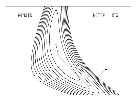
Fig. 10.12: Minimization in the direction of steepest descent.
