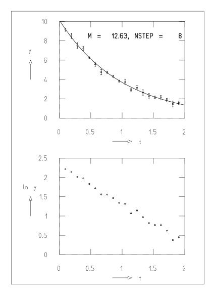
**Fig. 9.6:** Measured values and fitted exponential function (*above*); logarithms of the measured values (*below*).
