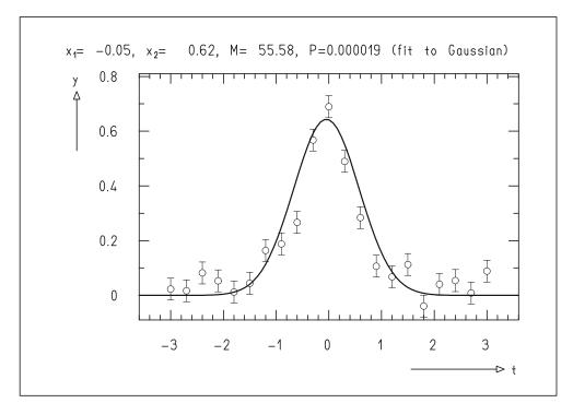
**Fig.G.12:** Fit of a Gaussian to data points that correspond to a Breit–Wigner function. The goodness-of-fit is poor.
