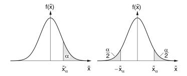
**Fig. 8.1:** One-sided and two-sided tests
