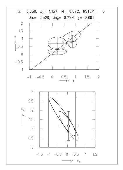
**Fig. 9.15:** (*Above*) Measured points with covariance ellipses and fitted line. (*Below*) Result of the fit, given in the plane spanned by the parameters  $x_1$ ,  $x_2$ . Shown are the fitted parameter values (*circle*), symmetric errors (*crossed bars*), covariance ellipse, asymmetric errors (*horizontal* and *vertical lines*), and the confidence region (*dark contour*).
