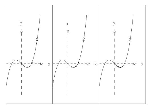
**Fig. 10.4:** Bracketing of a minimum with three points a, b, c according to (10.4.3). The initial values are shown as *larger circles*, and the results of the individual steps are shown as *small circles*.
