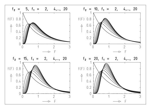
**Fig. 8.2:** Probability density of the *F*-distribution for fixed values of  $f_1 = 2, 4, ..., 20$ . For  $f_1 = 2$  one has  $f(F) = e^{-F}$ . For  $f_1 > 2$  the function has a maximum which increases for increasing  $f_1$ .
