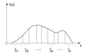
**Fig. 8.7:** Dividing the range of the variable x into the intervals  $\xi_k$ .
