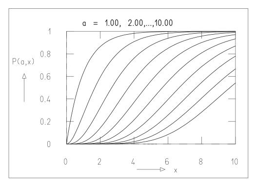
**Fig. D.3:** The incomplete gamma function. With increasing a the graphs P(a, x) move to the right.
