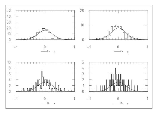
**Fig. 6.2:** Histogram of the same sample from a Gaussian distribution represented with four different bin widths.
