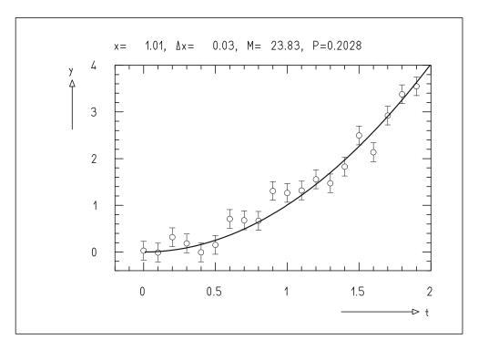
**Fig. G.10:** Result of the fit of a parabola  $y = xt^2$  to 20 measured points.
