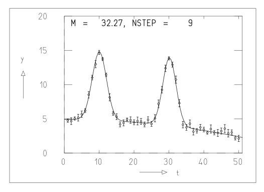
**Fig. 9.8:** Measured values and fitted sum of a second-order polynomial and two Gaussian functions.
