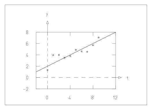
**Fig. 4.7:** Line in the (t, y)-plane and simulated measured values with errors in y.
