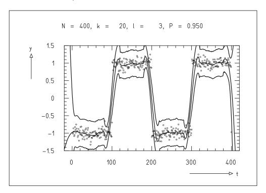
**Fig. G.16:** Time series corresponding to a step function with moving averages and confidence limits.
