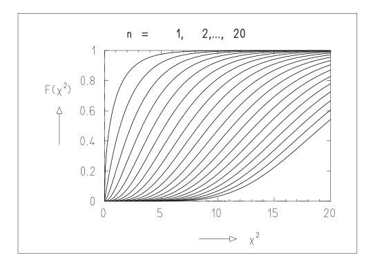
**Fig. 6.9:** Distribution function for  $\chi^2$  for the number of degrees of freedom n = 1, 2, ..., 20. The function for n = 1 is the curve at the far left, and the function for n = 20 is at the far right.
