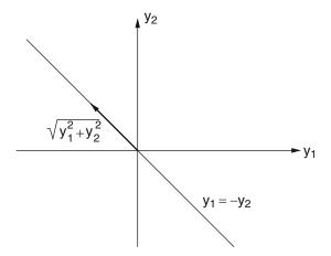
**Fig. 6.7:** A sample of size two gives a sum of squares with one degree of freedom.
