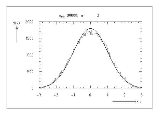
**Fig. G.6:** Histogram of 90 000 random numbers **x**, each of which is a sum of three uniformly distributed random numbers. The curve corresponds to the standard normal distribution. Significant differences between curve and histogram are visible only because of the very large number of random numbers used.
