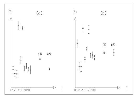
**Fig. 9.1:** Averaging of 10 measurements where the  $\chi^2$ -test fails. (a) Anomalous deviation of certain measurements: (1) Averaging of all measurements; (2) averaging without  $y_4$  and  $y_6$ . (b) Errors of individual measurements clearly too small: (1) Error of the mean according to (9.1.10); (2) error of the mean according to (9.1.13).
