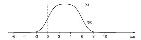
Fig. 5.16: Convolution of a uniform and Gaussian distribution.
