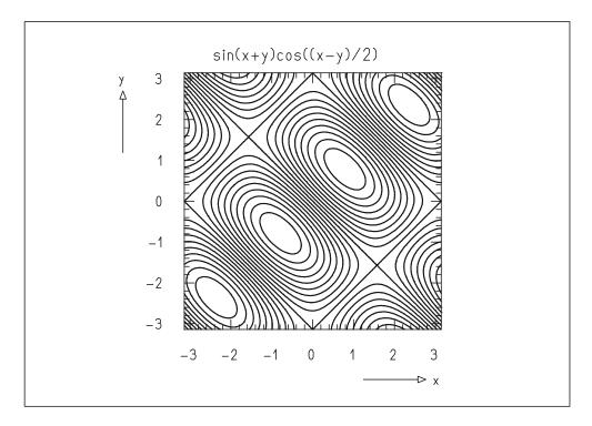
**Fig. F.5:** Contour lines f(x, y) = -0.9, -0.8, ..., 0.8, 0.9 of the function  $f(x) = \sin(x + y) \cos([x - y]/2)$  in the (x, y) plane.
