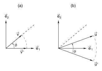
**Fig. A.4:** Application of the Givens transformation (a) to the vector **v** that defines the transformation and (b) to an arbitrary vector **u**.
