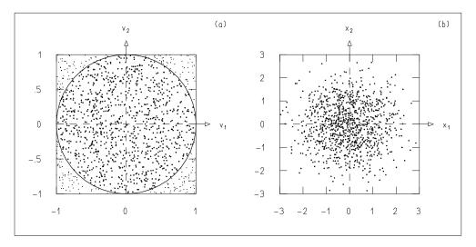
**Fig. 4.6:** Illustration of the Box–Muller procedure. (a) Number pairs  $(v_1, v_2)$  are generated that uniformly populate the square. Those pairs are then rejected that do not lie inside the unit circle (marked by *small points*). (b) This is followed by the transformation  $(v_1, v_2) \rightarrow (x_1, x_2)$ .
