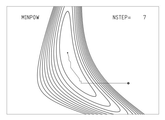
Fig. 10.11: Minimization along a chosen direction with the method of Powell.
