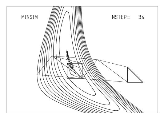
**Fig. 10.9:** Determining the minimum of a function of two variables with the simplex method. The function is shown by *contour lines* on which the function is constant. The function is highest on the outermost contour. The minimum is at the position of the *small circle* within the innermost contour. Each simplex is a *triangle*. The initial simplex is marked by *thicker lines*.
