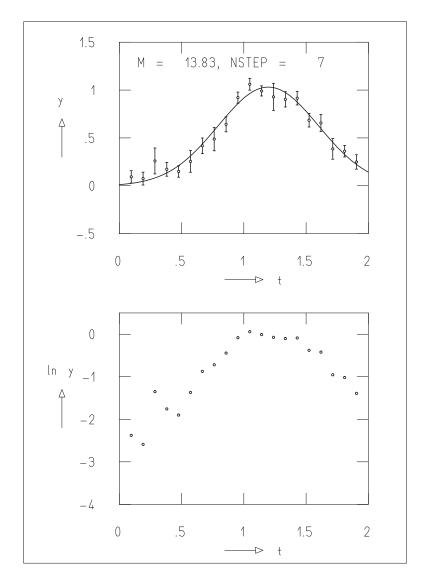
**Fig. 9.5:** Measured values and fitted Gaussian curve (*above*); logarithm of the measured values (*below*).
