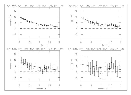
**Fig. 9.10:** Fit of an exponential function  $\eta = x_1 \exp(-x_2 t)$  to measurements with errors of different sizes.
