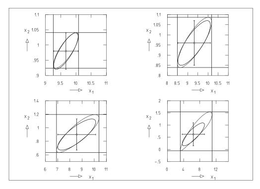
**Fig. 9.11:** Results of the fit from Fig. 9.10 in the parameter space  $x_1$ ,  $x_2$ . Solution  $\tilde{\mathbf{x}}$  (*small circle*), symmetric errors (*error bars*), covariance ellipse, asymmetric error limits (*horizontal* and *vertical lines*), confidence region corresponding to the probability of the covariance ellipse (*dark contour*).
