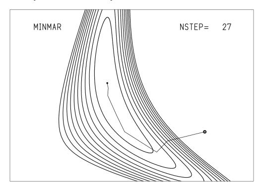
Fig. 10.15: Minimization with the Marquardt procedure.
