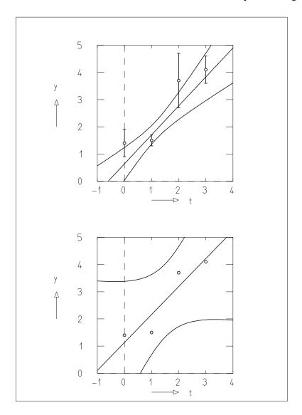
**Fig. 12.1:** (*Above*) Measurements with errors and regression line with 95% confidence limits. (*Below*) Measured points with errors assumed to be of unknown but equal magnitude, regression line, and 95% confidence limits.
