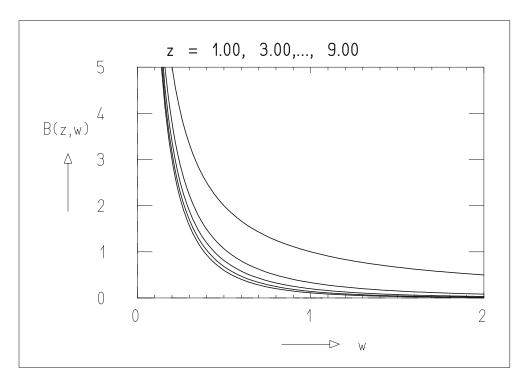
**Fig. D.2:** The beta function. For increasing z the curves B(z, w) are shifted to the left.
