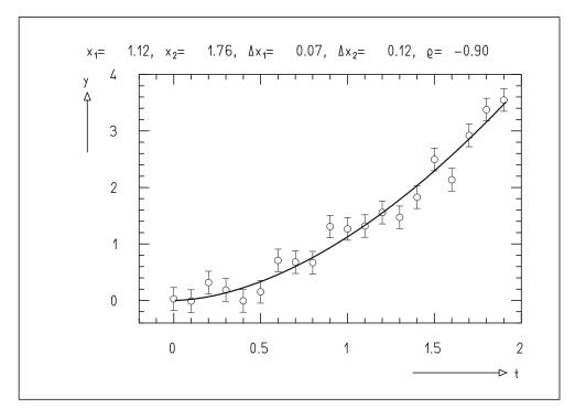
**Fig. G.11:** Fit of a function  $y = x_1 t^{x_2}$  to 20 data points. The data points are identical to those in Fig. G.10.
