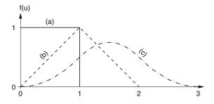
Fig. 5.15: Convolution of uniform distributions. Probability density of the sum u of uniformly distributed random variables x (a) u = x, (b) u = x + x, (c) u = x + x + x.
