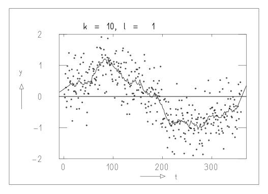
**Fig. 13.1:** Data points (*circles*) and moving average (joined by line segments).
