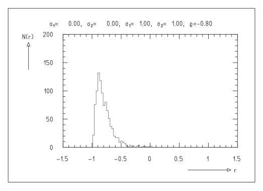
**Fig. G.8:** Histogram of the sample correlation coefficient computed for 1000 samples of size 10 from a bivariate Gaussian distribution with the correlation coefficient  $\rho = -0.8$ .
