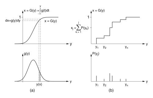
**Fig. 4.4:** Transformation from a uniformly distributed variable x to a variable y with the distribution function G(y). The variable y can be continuous (a) or discrete (b).
