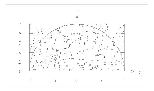
**Fig. 4.5:** All the pairs  $(y_i, u_i)$  produced are marked as points in the (y, u)-plane. Points above the curve u = g(y) (*small points*) are rejected.
