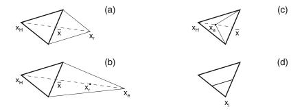
**Fig. 10.8:** Transformation of a simplex (*triangle* with *thick border*) into a new form (*triangle* with *thin border*) by means of a reflection (**a**), stretching (**b**), flattening (**c**), and contraction (**d**).
