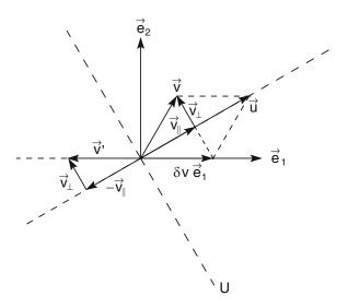
**Fig. A.5:** The vector  $\mathbf{v}$  is mapped onto  $\mathbf{v}'$  according to a Householder transformation such that  $v_2' = 0$ . The mapping corresponds to a reflection in the subspace U that is orthogonal to the auxiliary vector  $\mathbf{u}$ .
