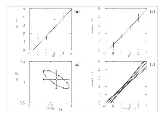
**Fig. 9.2:** Fit of a *straight line* to data from Table 9.2. (a) Original measured values and errors; (b) improved measurement values and residual errors; (c) covariance ellipse for the fitted quantities  $x_1, x_2$ ; (d) *various lines* corresponding to individual points on the covariance ellipse.
