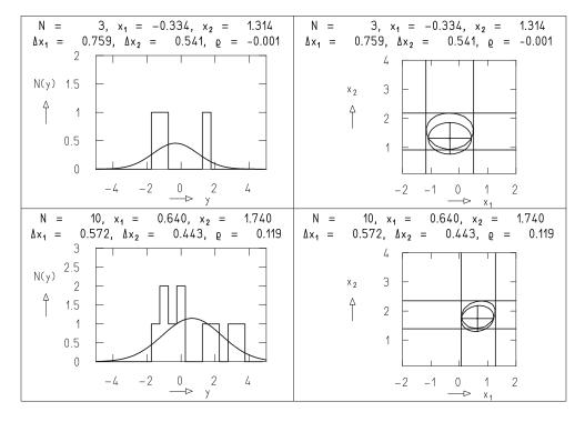
**Fig. 10.17:** Determination of the parameters  $x_1$  (mean) and  $x_2$  (width) of a Gaussian distribution by maximizing the log-likelihood function of a histogram. The *left-hand plots* show two histograms corresponding to the samples from Fig. 10.16. The curves are the Gaussian distributions normalized to the histograms. The *right-hand plots* show the symmetric errors, covariance ellipse, and confidence region represented as in Fig. 10.16.
