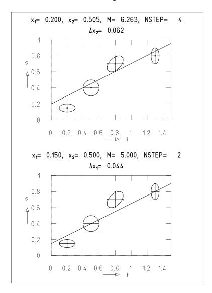
**Fig. 9.13:** Fitting a line to the same points as in the first plot of Fig. 9.12. The intercept with the vertical axis  $x_1$  was held constant in the *upper plot*, and below the slope  $x_2$  was held constant.
