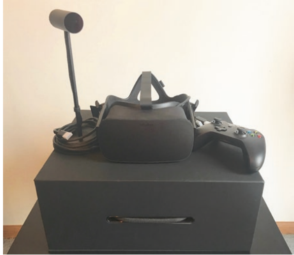
Fig. 5 Oculus Rift sensor, headset, and Xbox controller (from left to right)
